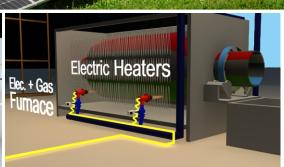
**Solar Power** can be directly(DC supply) used for **Heating Furnaces** during daytime. These furnaces are also fitted with Automatic gas burners. As solar energy reduces, gas heating starts. Solar retakes over next day morning. This combination of **SOLAR+GAS** reduces operating cost up to 60% compared with Government Power supply tariff. The Cost of Investment is recovered in less than a year or even less if 100% depreciation is availed.
